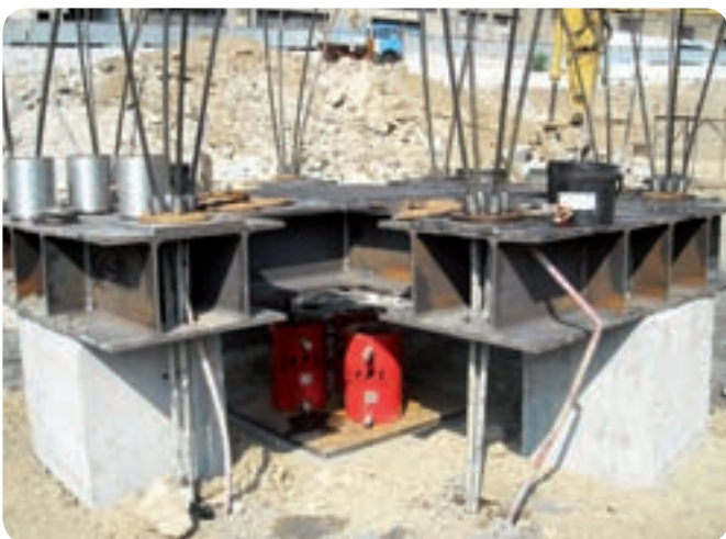
Load tests on foundation piles and failure recording with 250 ton-capacity, 250 mm stroke F.P.T. cylinders - model CRI250/250
