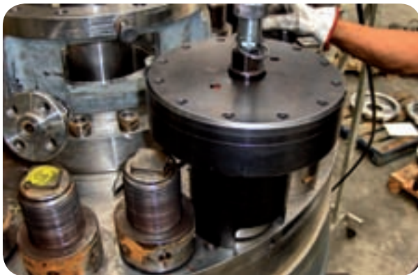
M64x4 120-ton capacity hydraulic tensioner with spring to return the piston.
