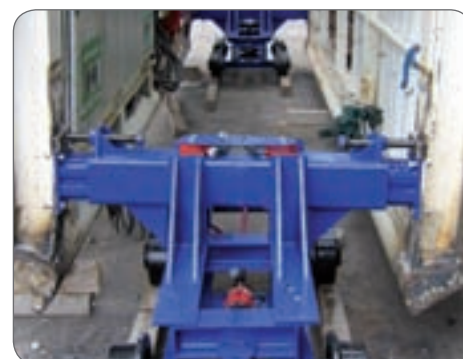
Equipment to support decks in tunnels consisting of a PMSA 3.5 pump and 10-ton cylinders.
