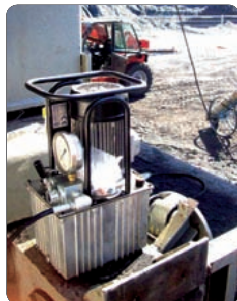
Electric control unit for lifting a roupelle.
