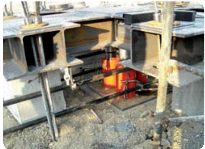
Load tests on foundation piles and failure recording with 250 ton-capacity, 250 mm stroke F.P.T. cylinders - model CRI250/250
