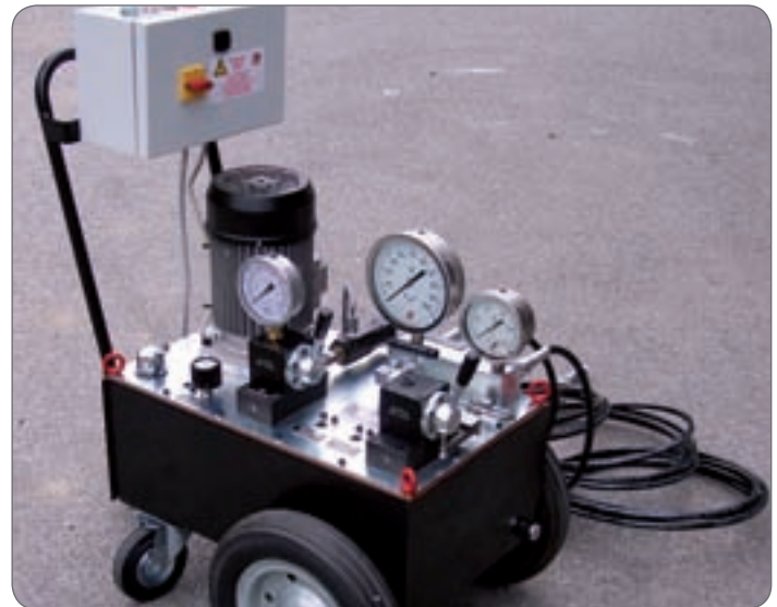
Hydraulic pump to operate strand tensioning cylinders in the field of post-tensioning
