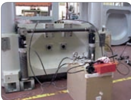
Pump with 8-litre reservoir for lifting a press section.
