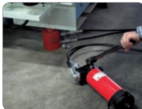
PDSA20 DE pump to operate a double-acting cylinder to level large machinery.
