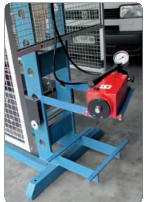
Two-speed pump to operate both the single and double-acting press cylinder.
