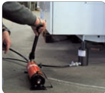
CSE 50/100 for lifting machinery.
