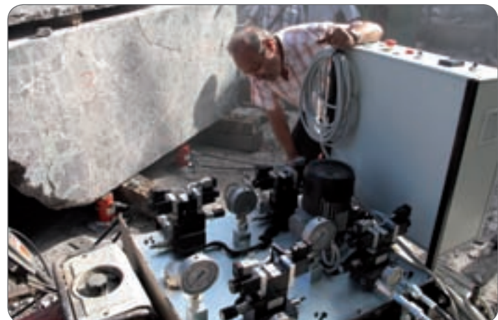
Hydraulic pump with 4 independent outlets for synchronous lifting of the load, independently from the different load weighing on each cylinder.
