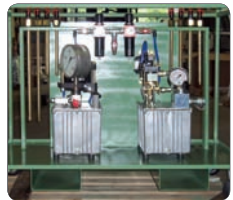
Unkeying unit with double pneumohydraulic unit (700 bar and 3000 bar).
