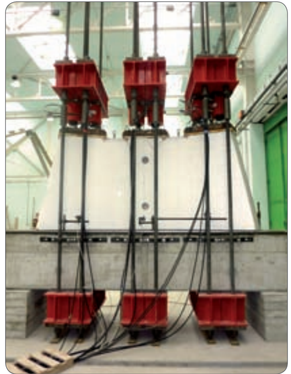
Compression tests in a civil engineering laboratory with 200-ton CRIC cylinders.
