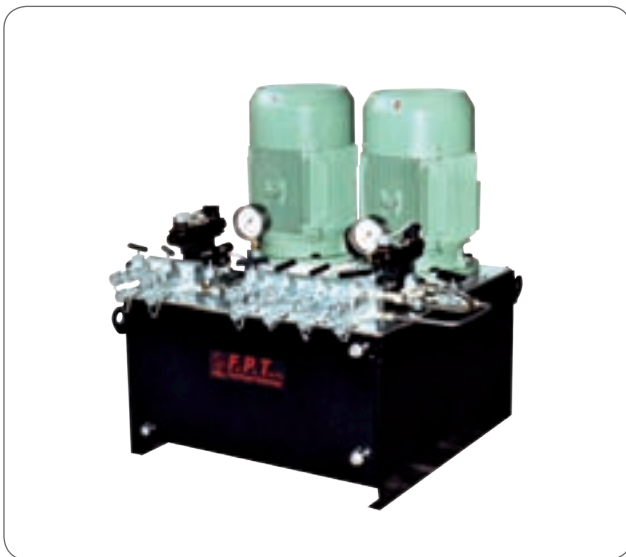
Hydraulic pump, equipped with an inverter on both motors for acceleration and deceleration ramp control, to operate 2 separate groups of cylinders.
