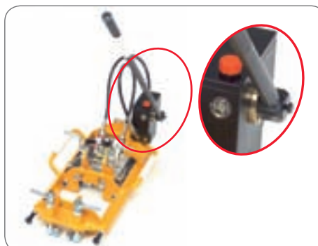
Pump with 2 pumping pistons for bidirectional operation to pump in both handle stroke directions. Built for railway applications.
