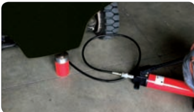
Maintenance on earth-moving machinery and workshop machines – 30-ton cylinder with spring return.
