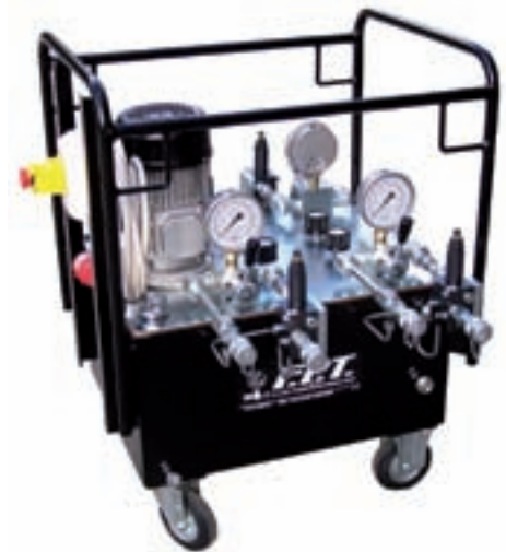
Hydraulic pump with 4 independent delivery ports with single overcentre valves (700 bar) to synchronise the load in both lifting and lowering.
