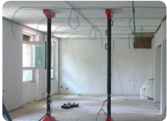
Hydraulic kit for floor Load Tests, used to carry out static load tests with concentrated load. Kit comprising support cross members, hydraulic cylinder, light alloy extensions and hydraulic pump
