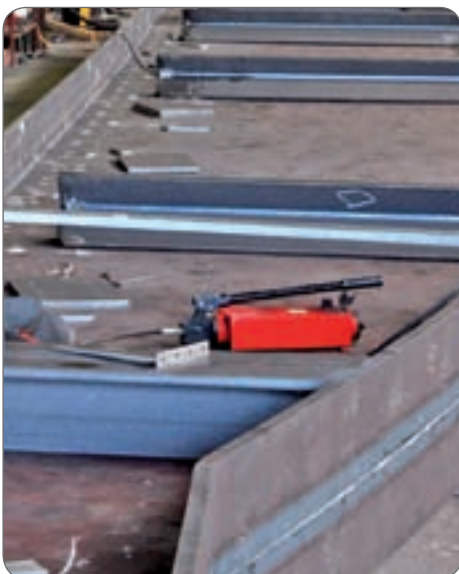
Hand pump for placing structural steelwork on a jig.
