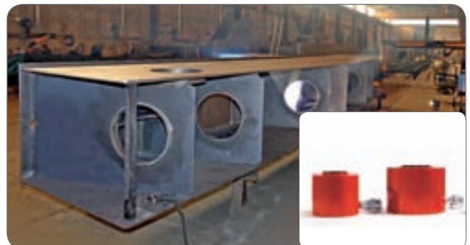
Compact cylinder with spring return (50-ton capacity) used for heavy structural steelwork.
