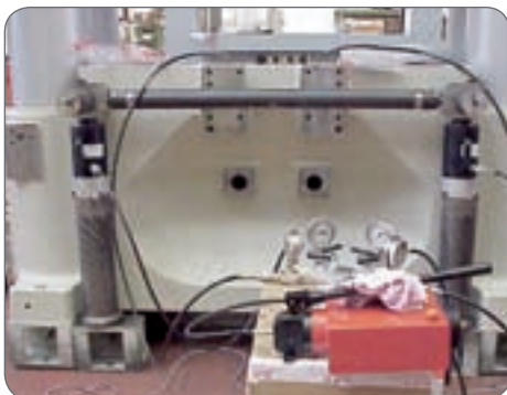
CRMA 50/150 to lift a press section.
