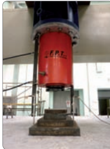
400-ton CRI cylinder and hydraulic pump for load tests on reinforced concrete structures.
