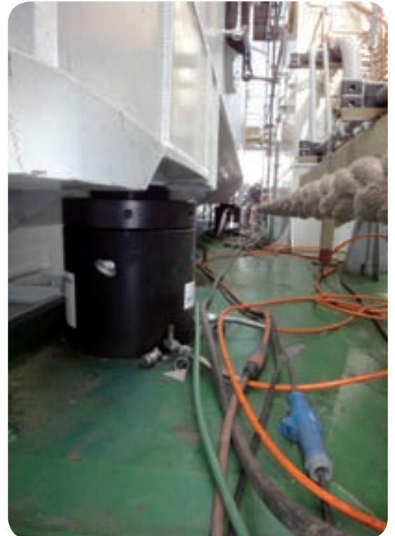
4 high-tonnage double-acting cylinders, with 600 ton-capacity 250 mm flow mechanical locking ring, controlled by 2 F.P.T. hydraulic pumps.
