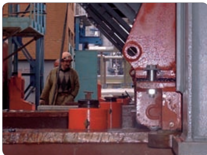
Compact cylinder with spring return (100-ton capacity and 50 mm stroke) and self-levelling head.
